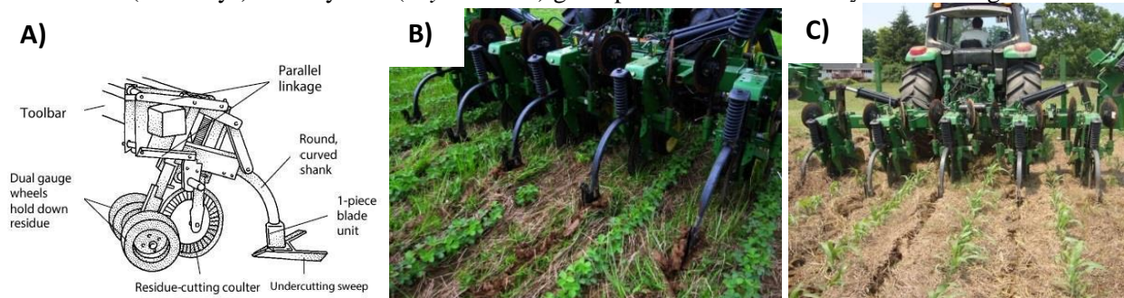
Figure 1. High Residue Cultivators. A) High residue cultivator schematic (from North Carolina State University), B) in organic soybean production, and C) in conventional no-till corn production
