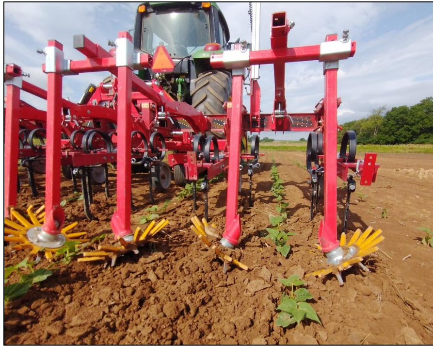
Figure 1. Cultivator setup using camera guidance to direct finger-weeder cultivators at V1-2 crop growth stage.
